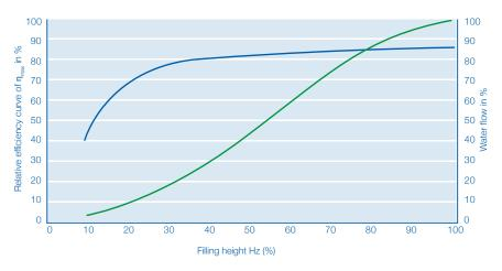
Blue Line – indicates the efficiency (relationship between power fed in and power passed on) measured according to the water flow pumped.
