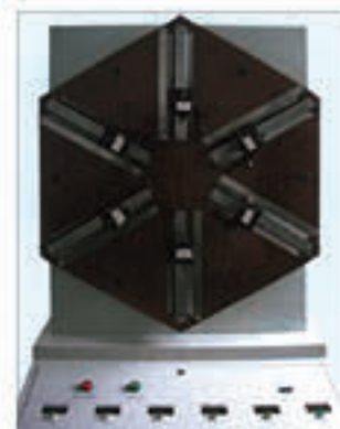
Performance Test Station of Tubular Conveyor Belt
