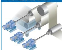
Many geared motors are used at rollers in aggressive environments like galvanising, annealing or coating lines.
