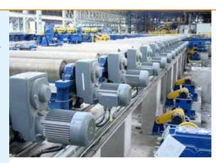
Parallel shaft geared motors for roller tables
