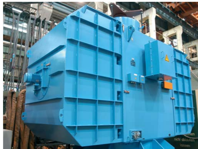
Pump drive High-voltage asynchronous motor with squirrel-cage rotor 2,550 kW / 6,000 V / 331 rpm
