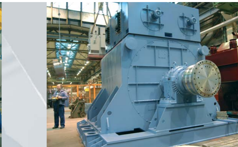
Rolling mill drive High-voltage synchronous motor 5,000 kW / 2,000 V / 0-160 / 400 rpm
