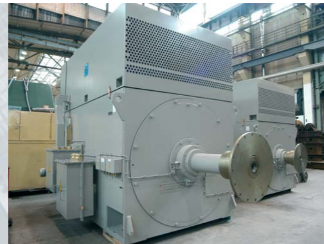
Mill drive Three-phase asynchronous motor with slipring rotor 4,000 kW / 11,000 V / 994 rpm
