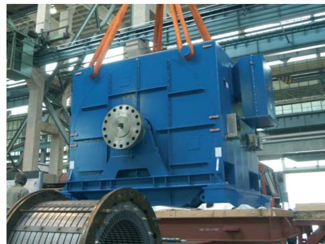
Compressor drive High-voltage synchronous motor Ex p II BT3 7,600 kW / 10,000 V / 360 rpm
