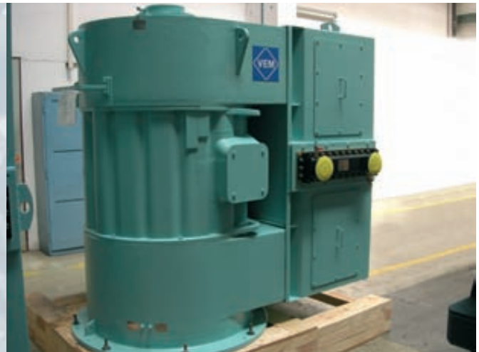
Project "Cruiseliners AIDA I-VI" , Meyer Shipyard / Germany DKKJT 7124-8WF 2,300 kW, 11,000 V, 900 r.p.m., IM 4011, IC 8A1W7
