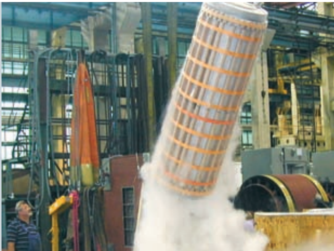
Project "Schottel SEP-5", Royal Schelde Yard/Netherlands DKWUZ 9088-12V 5,500 kW, 3,300 V, 212 r.p.m., IM 5009
