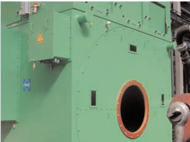
Project "container ship for Hapag Lloyd", HHI shipyard/Korea DGMUX 1645-16W 5,000 kVA, 6.400 V, 65 – 94 r.p.m., IM 5406, IC 8A6W7
