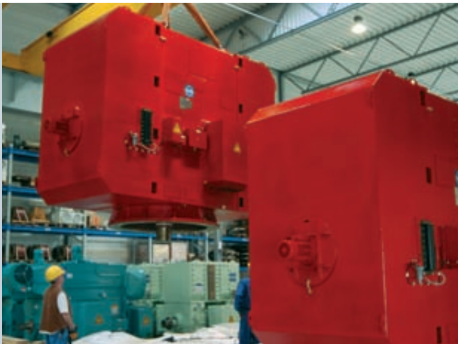
Project "Pipe fitter ship Solitaire" DTMTZ 9038-6Y 4,300 kW, 2 x 1.250 V, 465 r.p.m., IM 3011, IC 8A6W7
